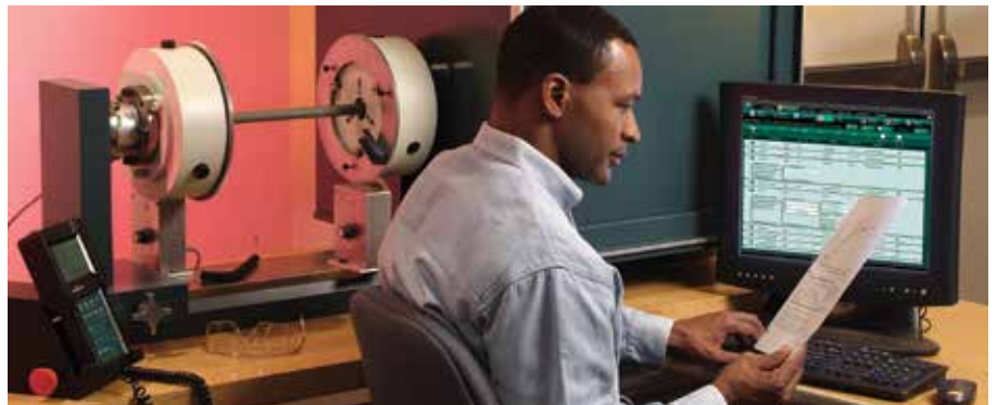
Fig 2. Bench mounted 10,000 in.lbf machine.
