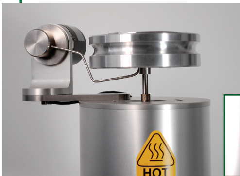
Fig 4. New design of tapered weights, for safer loading and unloading.
