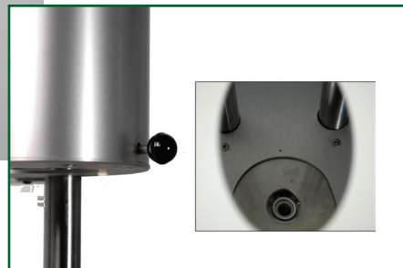
Fig 3. Close-up showing die release knob and inset, looking in mirror at the die.
