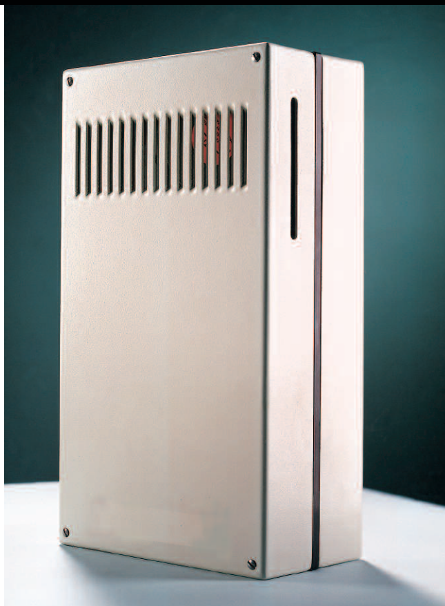
Fig. 1. Model 500LC scanning laser extensometer.
